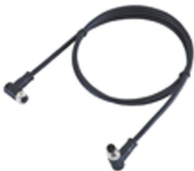
M8 6Pin male to female, right angled, molded 6x26AWG PVC cable
